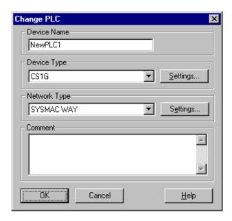
Enter PLC's name in the project (e.g. default name NewPLC1), PLC's model (e.g. CS1G) and set the communication type used to access the configured PLC (SYSMAC WAY - for serial communication).
